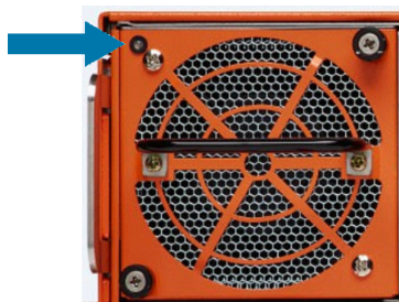
Figure 6 Individual Fan LED Location on GigaVUE-HC3 Rear
